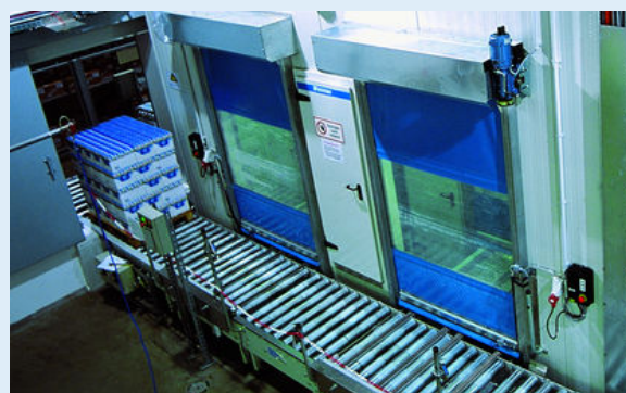
Tunnel cooler – chilling of yogurt from 20/25 °C down to 6 °C, 50 pallets per hour
